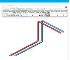
Design sigle or multiple pipes turn by turn, specifying points on the drawing...
